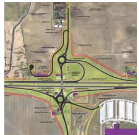
At a new interchange in Tipton County, State Road 28 bridges over U.S. 31 and has single-lane roundabouts designed to accommodate agricultural equipment, large trucks, and future expansion. The design also includes direct access to the Tipton Transmission Plant and a looping ramp for traffic entering southbound U.S. 31.
